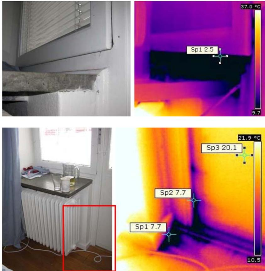
The air-leakage is mostly due to poor sealing's in and around windows and balcony-doors.
