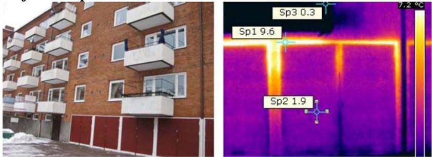
The upper picture shows the normal heat-conduction from where joists and inner-walls meet the outer-wall. In the same picture we see the affect of a window not quite shut. The lower picture shows the heat-leakage from the garage doors.
