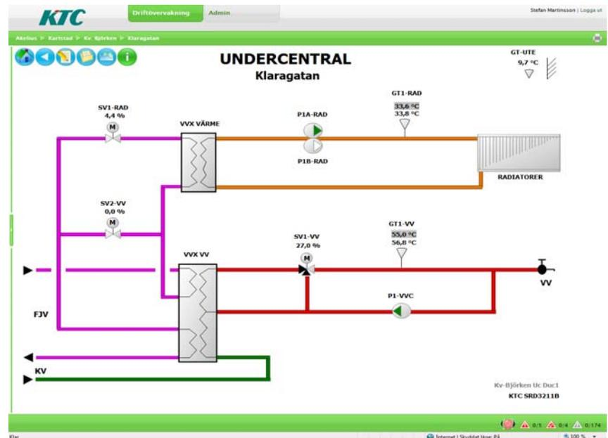
**Picture 3. Monitoring heating and hot water**
