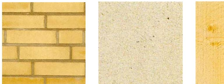
The more compact a construction material is, the less air it can store up. The lesser the non circulating air, the poorer the insulation. A brick wall must be five times as thick, and a lightweight concrete wall twice as thick as a wooden wall in order to give the same insulating effect.
