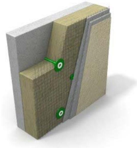
*Example of insulation with new trimmed facade*
