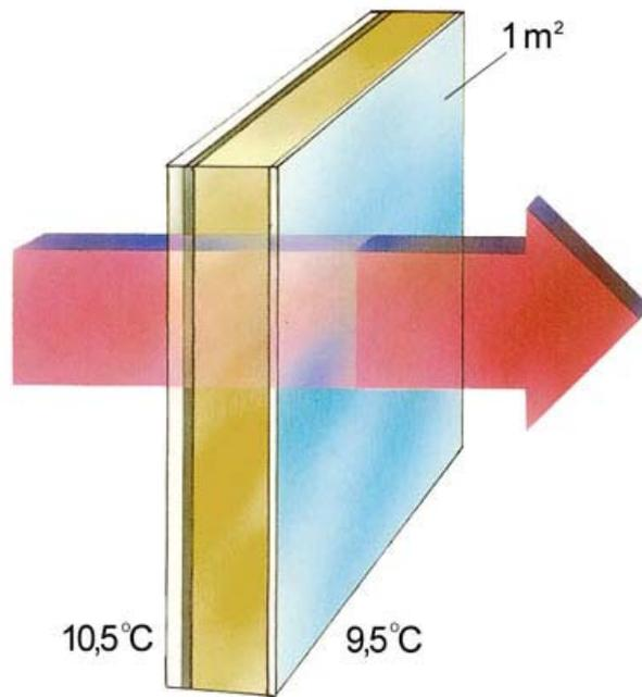
*Example a wall with U-Value of 1.0 W/m<sup>2</sup>k, means that the wall loses 1.0 Watt in this condition*
