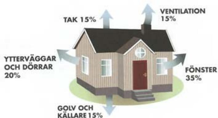
*Examples of heat losses: Floors 15 %, Windows 35%, Walls 20 %, Roof 15 % and ventilation 15 %*
